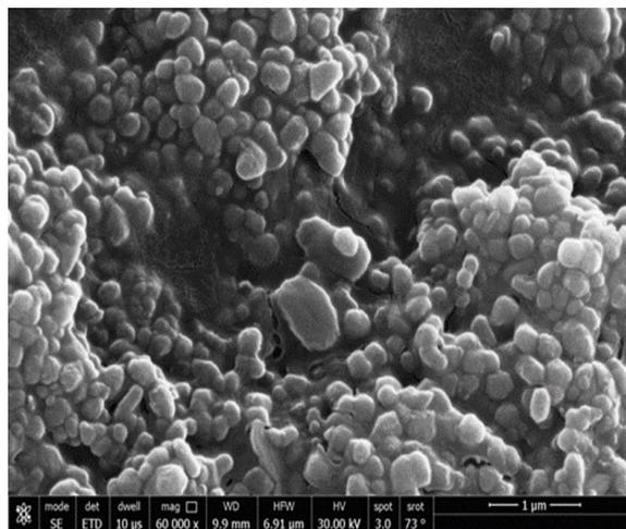
Fig. 2. Illustrate the spherical monodispersed ZnO-NPs SEM image.
