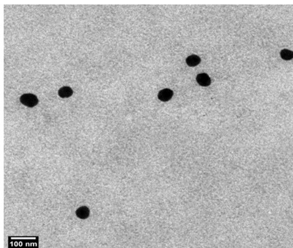
Fig. 3. Illustrate the TEM image of ZnO-NPs nanospheres.
