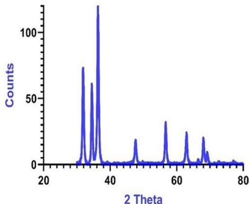
Fig. 1. Illustrates the fingerprint of XRD pattern of ZnO NPs according to Brucker database COD no. 2300113.
