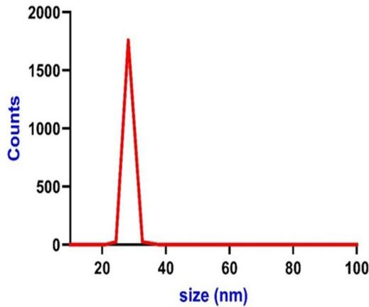
Fig. 4. The DLS pattern of ZnO NPs.
