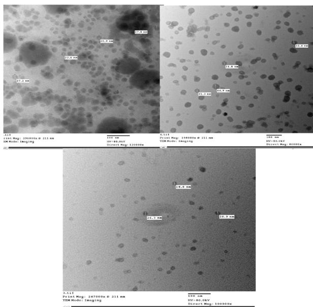
Fig. 2. Transmission electron microscopy (TEM) images of the synthesized CaO-NPs displaying particle size distribution.
