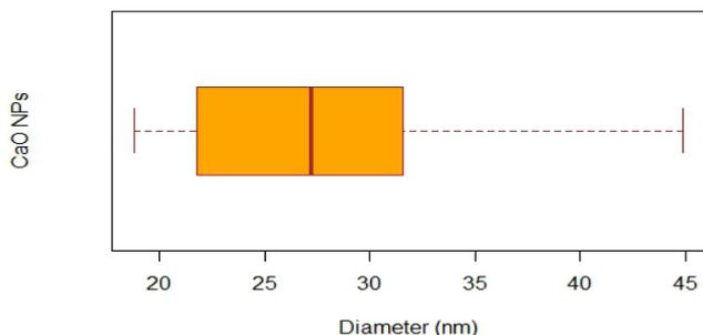
Fig. 3. Diameter range of the synthesized CaO-NPs measured by TEM.
