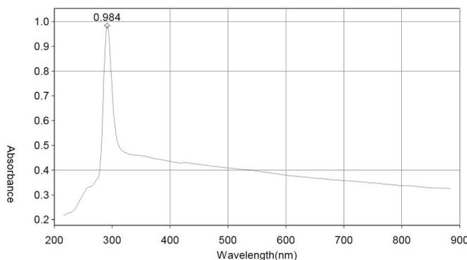
Fig. 5. Ultraviolet-visible (UV-Vis) spectroscopy spectrum of the synthesized CaO NPs.
