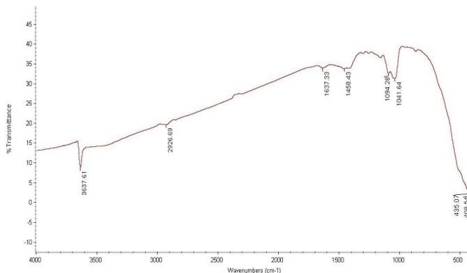
Fig. 4. Fourier transform infrared spectroscopy (FTIR) spectrum of synthesized CaO-NPs. The mid-infrared spectrum (wavenumbers cm<sup>-1</sup>) were plotted on the horizontal axis between 4,000 and 400 cm<sup>-1</sup>, while the peaks (absorbance bands) represent the different vibrations of the material's atoms. The vertical axis identifies the quantity of infrared light transmitted by the analyzed nanoparticle material.
